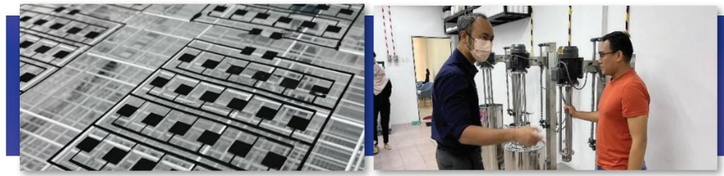
A sample of screen-printed conductive paste from SPT for touch panel application.
